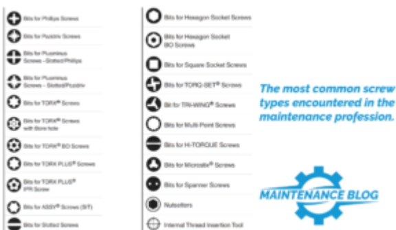
Common Screw Head Types
