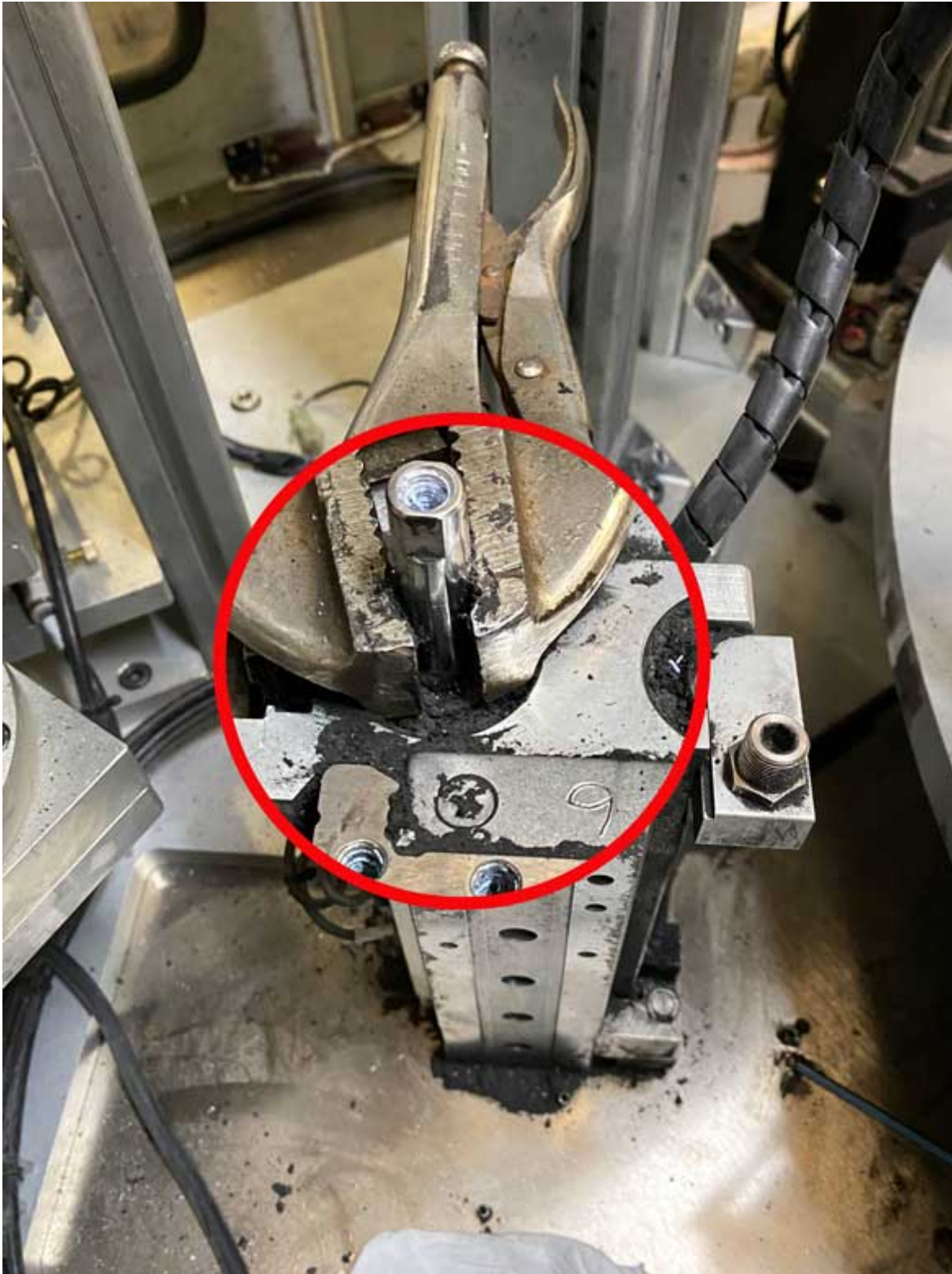
Vise Grips Causing Damage to an Air Cylinder Piston
