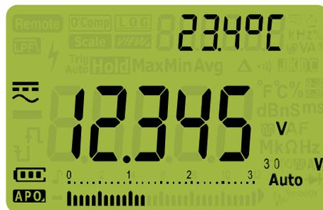
**Figure 2-7** AC+DC voltage display
