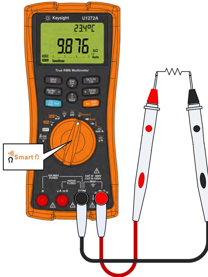
Figure 2-14 Measuring resistance
