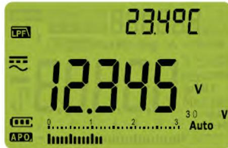
**Figure 2-8** Low Pass Filter(LPF) for AC+DC voltage measurements
