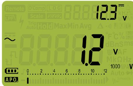
**Figure 2-11** Z<sub>LOW</sub> display
