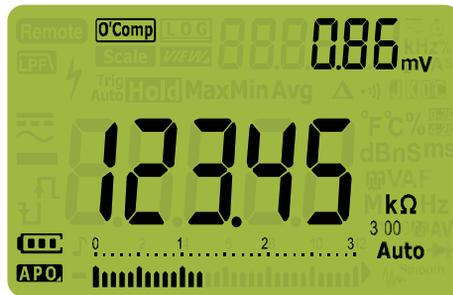
**Figure 2-17** Smart  $\Omega$  (with bias voltage) display
