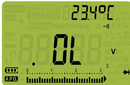
**Figure 2-20** Open diode display
