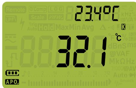
**Figure 2-27** Temperature display
