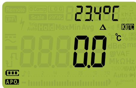
Figure 2-29 Temperature measurement without ambient compensation
