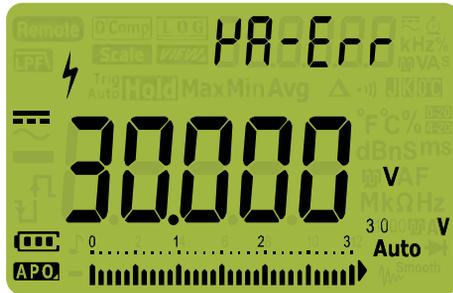
**Figure 1-3** Input warning display
