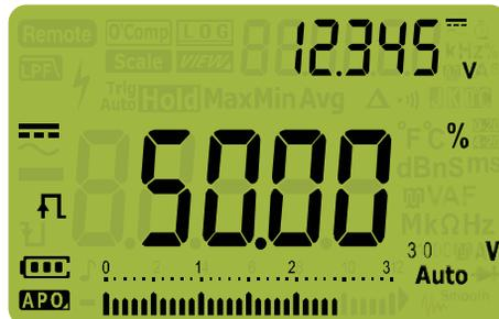
**Figure 2-40** Duty cycle display
