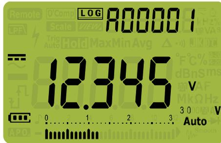
**Figure 3-7** Interval log display
