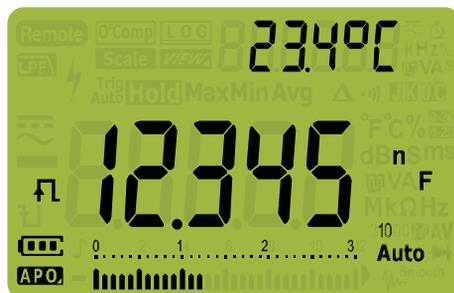
Figure 2-25 Capacitance display
