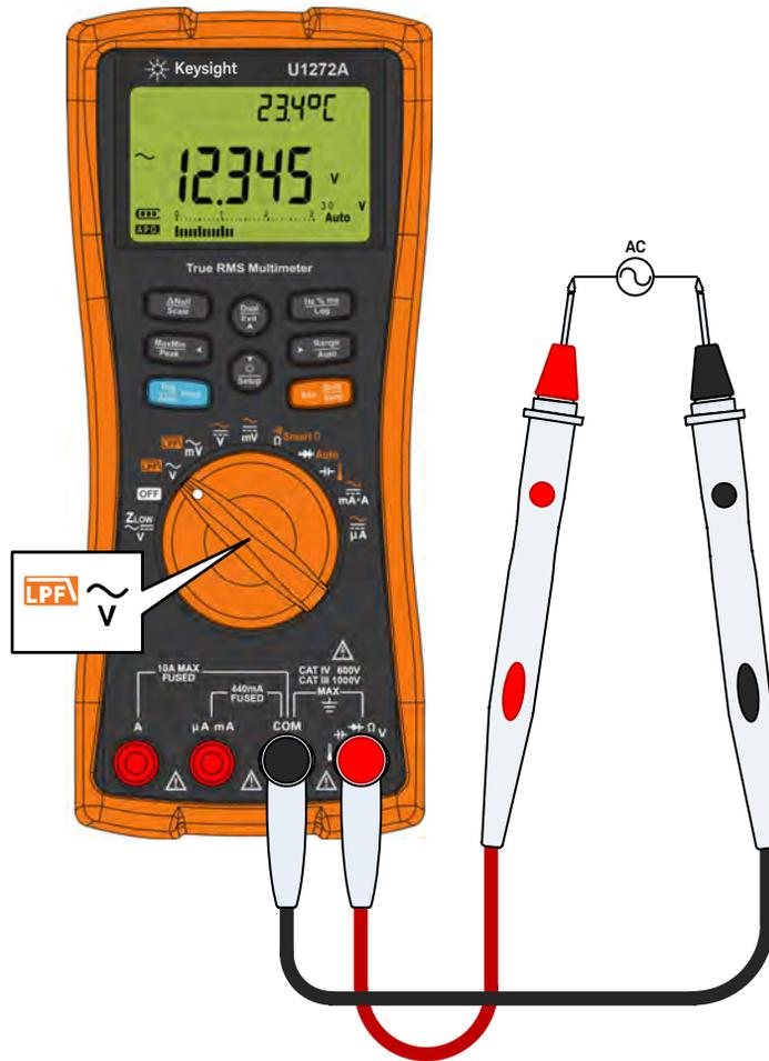
Figure 2-2 Measuring AC voltage
