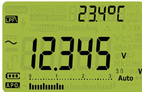
Figure 2-3 AC voltage with LPF display
