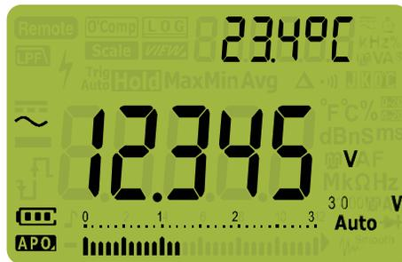
Figure 2-1 AC voltage display
