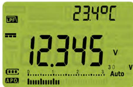
Figure 2-6 Filter for DC voltage measurements
