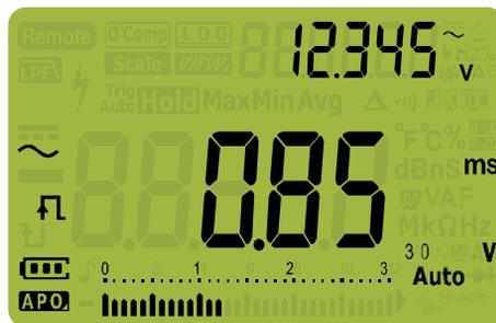
**Figure 2-39** Pulse width display
