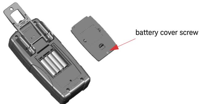
**Figure 4-1** Battery replacement
